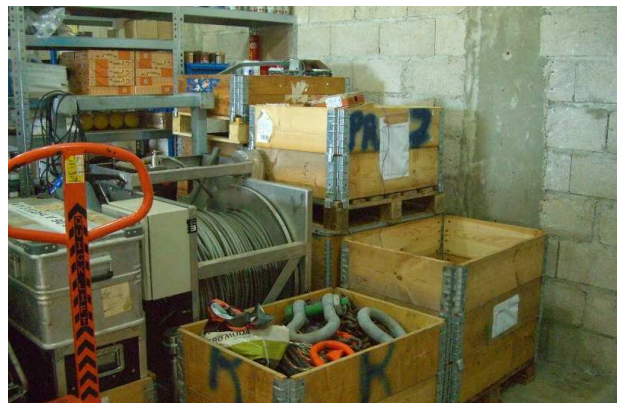
Figure 2-153: Electric Winch Stored in the Workshop (for a maximum lift of 9 tons)
