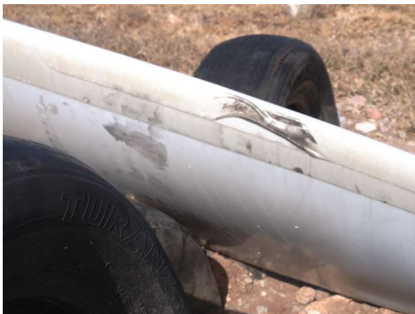
Figure 2-120: Blade Damage through Hoisting/Lowering
