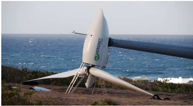
Figure 2-107: Access to Nacelle by Means of Ladders
