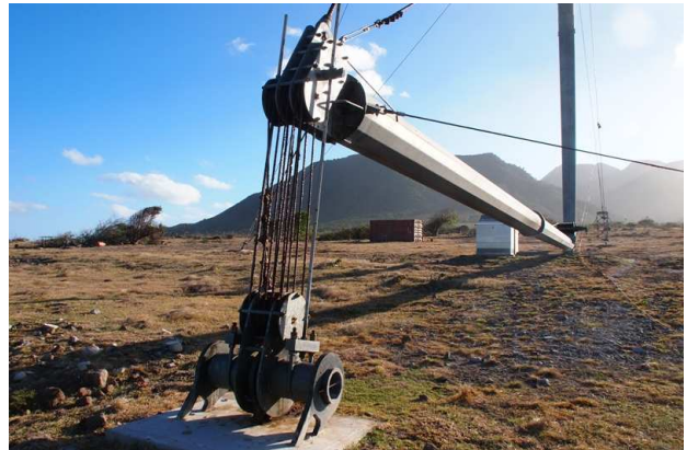
Figure 2-121: Gin Pole with Hoisting Mechanism
