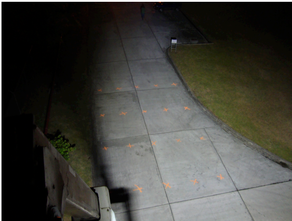
Figure 9: Evaluation pattern for illuminance tests, view from bucket truck
