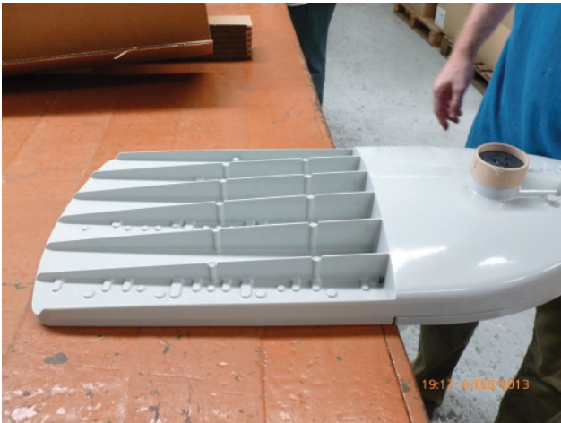
flat cooling device --> water cannot drain off
