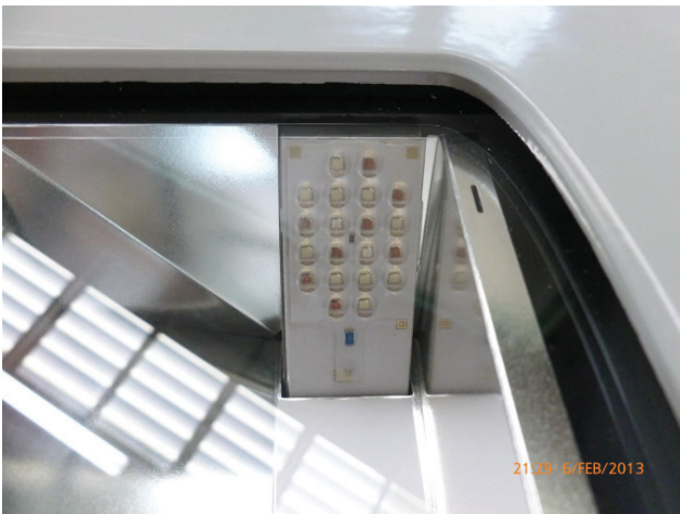
LED platines at the sides, Optic: reflector
