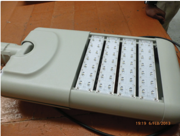
LED'S on different numbers of platines
