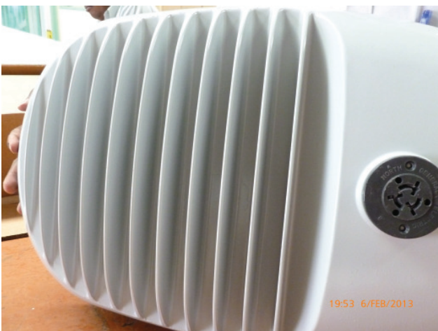
cooling device is flat, water collects in it
