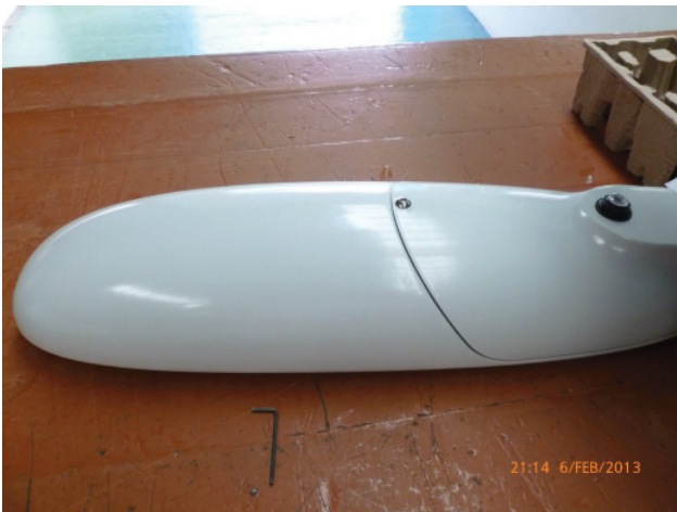
no cooling fin, heat conduction maybe over the whole body
