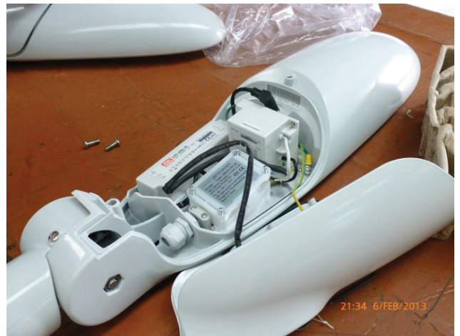
top cover fixed with a screw
