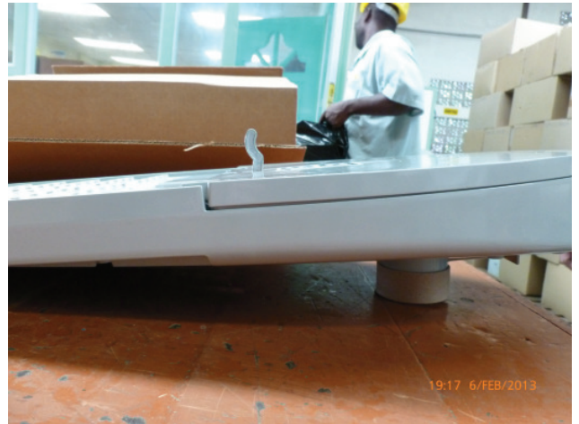
slot --> water can get easily into the luminaire
