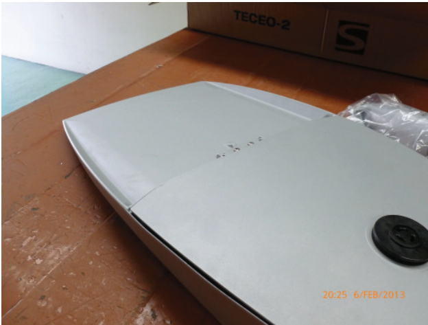
luminaire from the top, no visible cooling device
