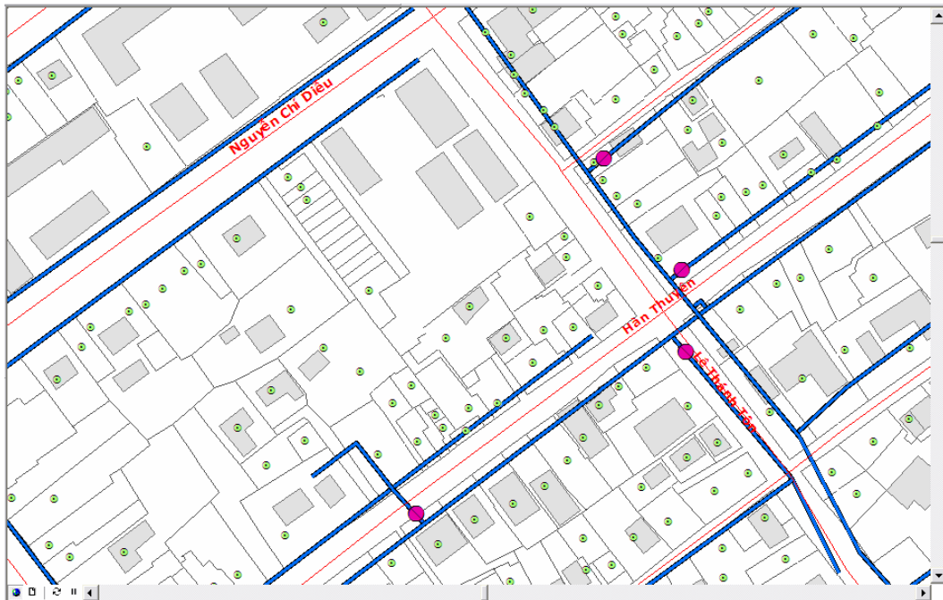
Figure 19: Registration of Wastewater network with Valves
